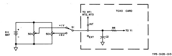
Frequency Adjustment Bias, Test Setup Figure 7
